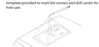
Use ø65mm hole saw to cut the hole, deburr and thoroughly clean surface with an alcohol wipe.
