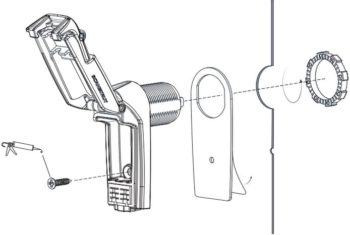
④ Connect to 12/24V supply, ensuring a waterproof connection. Fuse and select cable diameter according to input voltage and current for your specific installation.
