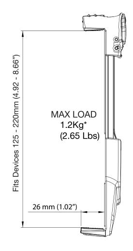
\*assuming product is installed in a dynamic environment where accelerations of up to 6g will be experienced
