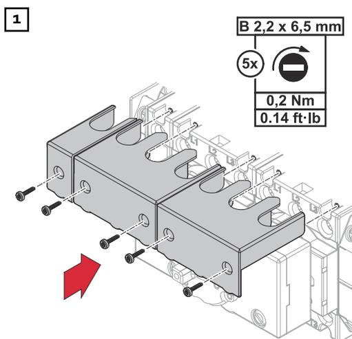
Mount a top protective cover on each of the load disconnectors 63 A. Fit using the screws supplied with the delivery.
