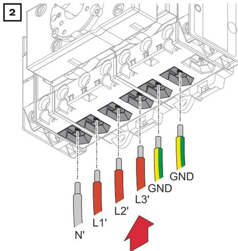
Plug the individual conductor (L1', L2', L3') coming from the backup power circuit and the neutral conductor (N') coming from the backup power circuit into the terminals. Plug the grounding cables (GND) of the house wiring into the terminals provided.
