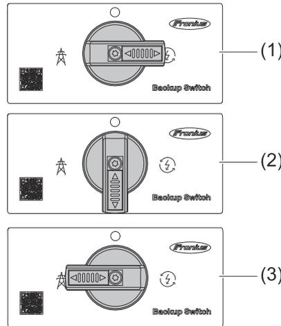
The backup switch has three switch positions:
