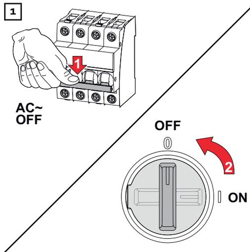
Turn off the automatic circuit breaker. Set the DC disconnecter to the "off" (OFF) switch position.
