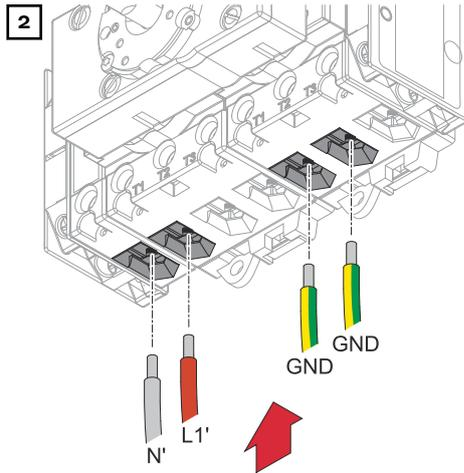
Plug the individual conductor (L1') coming from the backup power circuit and the neutral conductor (N') coming from the backup power circuit into the terminals. Plug the grounding cables (GND) of the house wiring into the terminals.
