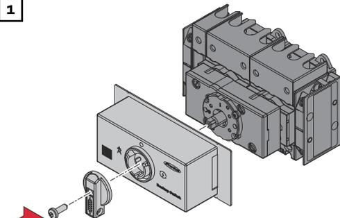
Install the housing cover and the switch and secure with the screw.
