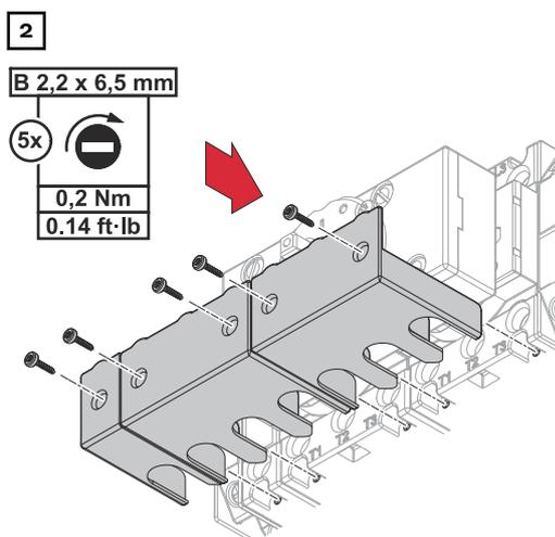
Mount a bottom protective cover on each of the load disconnectors 63 A. Fit using the screws supplied with the delivery.
