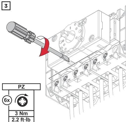
Screw the single conductors (L1', L2', L3') and the neutral conductor (N') into the terminals. Screw the grounding cables (GND) of the house wiring into the terminals.
