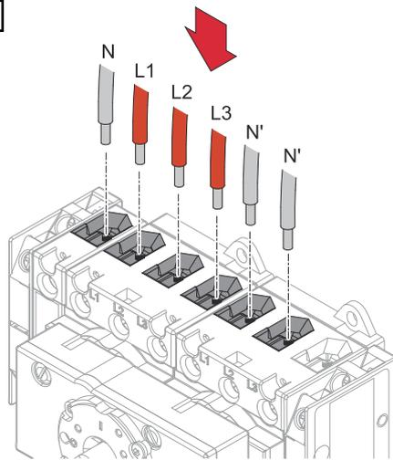
**3** Screw the single conductors (L1, L2, L3) and the neutral conductor (N) into the terminals. Screw the two neutral conductors (N') into the terminals. For permissible connection screws and torques, see **Permitted connection screws** on page **19**.
