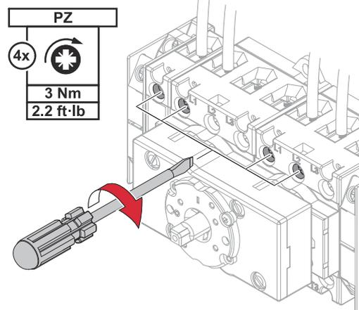
Screw the single conductor (L1) and the neutral conductor (N) into the terminals. Screw the two neutral conductors (N') into the terminals. For permissible connection screws and torques, see [Permitted connection screws](#) on page [19](#).
